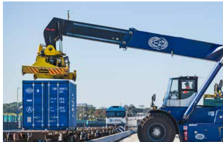
A reach stacker loads a train at Port Botany. Photo: NSW Ports
